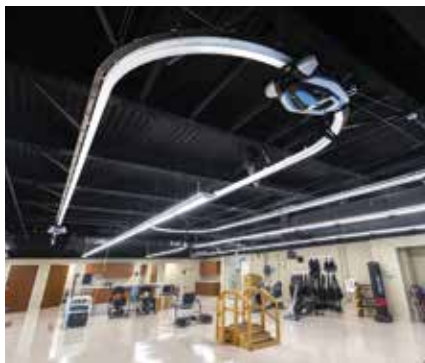
At the Cardinal Hill clinic, an overhead track system and harness supports patients as they work on walking, gait training and other physical skills.
